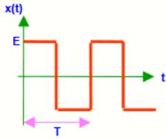
$$x(t) = \frac{4E}{\pi} \left[ \sin(\omega t) + \frac{\sin(3\omega t)}{3} + \frac{\sin(5\omega t)}{5} + \dots \right]$$
