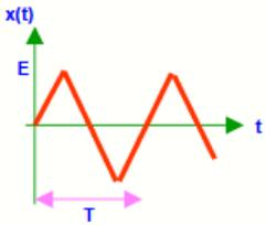
$$x(t) = \frac{8E}{\pi^2} \left[ \sin(\omega t) - \frac{\sin(3\omega t)}{3^2} + \frac{\sin(5\omega t)}{5^2} - \dots \right]$$
